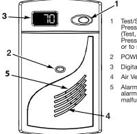
Test/Silence/Scroll Button: Press and release to select mode (Test, Memory, Clear Memory); Press and hold to activate mode, or to silence the alarm.
